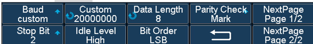
Figure 51 BUS CONFIG Menu
