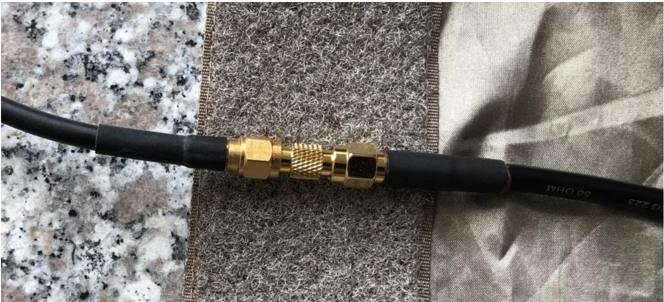
Picture 9: feed through using coaxial adapter
