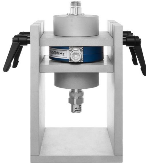
Picture 2: TBCP4-CAL RF current probe calibration fixture
