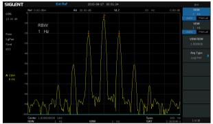
Phase noise -98 dBc/Hz@ 1 GHz, offset 10 kHz
