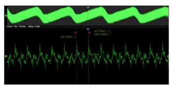
Utilizing a hardware-based Zoom technique and record length up to 200 Mpts, users can select a slower timebase without compromising the sample rate and then quickly zoom in to focus on the area of interest.
