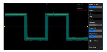
The SDS2000X Plus utilizes a hardware-based Mask Test function, performing up to 80,000 Pass / Fail decisions each second. It is easy to generate user defined test templates which the signal trace can be continuously compared to. The failed frames can be automatically stored as history frames or screen shots, making it suitable for long-term signal monitoring or automated production line testing.
