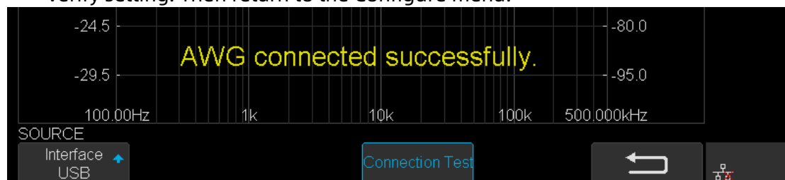
Figure 133 Bode Plot Interface Connection
