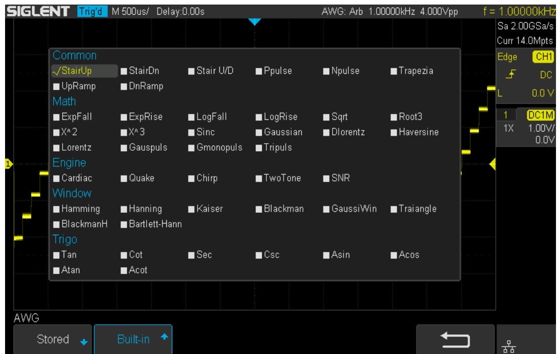
Figure 113 Built-in Arb interface
