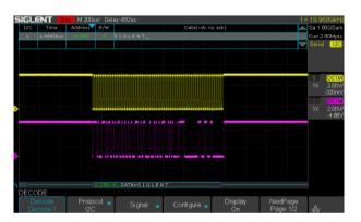
SDS2000X-E displays the decoding through the events list. Bus protocol information can be quickly and intuitively displayed in a tabular format.
