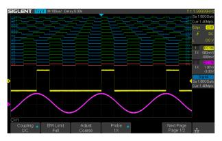
16 digital channels enables users to acquire and trigger on digital input channels and view both digital and analog waveforms simultaneously with one instrument.
