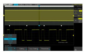
The SDS2000X-E can search events specified by the user in a frame. It can also navigate by time (delay position) and historical frames.
