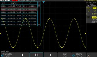
Playback the latest triggered events using the history function. Segmented memory collection will store trigger events into multiple (Up to 80,000) memory segments, each segment will store triggered waveforms and timestamp of each frame.
