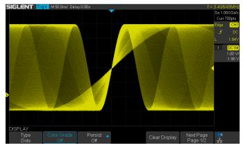
SPO display technology provides fast refresh rates. The resulting intensity-graded trace is brighter for events that occur with more frequency and dims when the events occur with less frequency.
