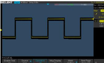
The SDS1000X-U utilizes a hardware-based Pass/Fail function, performing up to 40,000 Pass / Fail decisions each second. Easily generate user defined test templates provide trace mask comparison making it suitable for long-term signal monitoring or automated production line testing.
